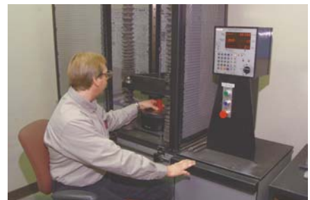
Computer Controlled Spring Testing - Utilizing custom software, spring testers track and verify consistency in spring dimensions and rates.
